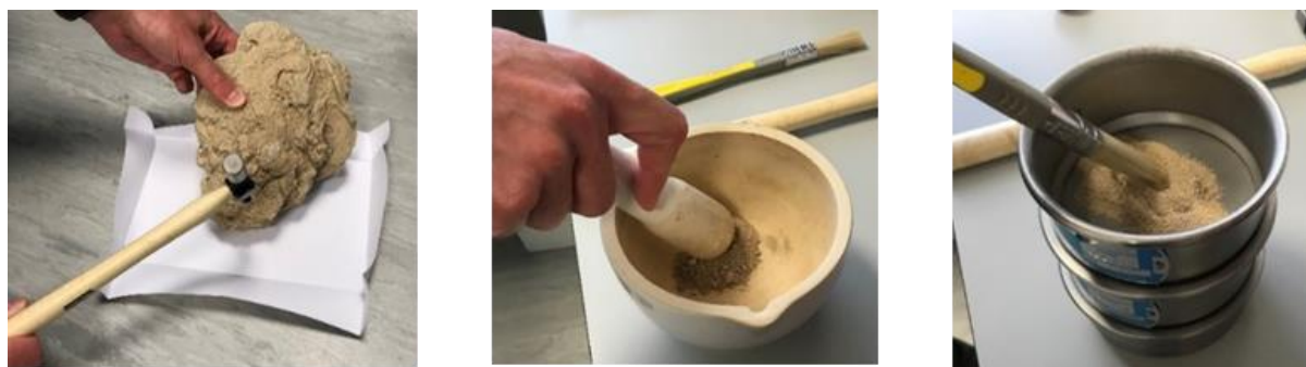
Figure 1. Preparation of mortar sample for analysis: subsamples are removed from the initial lump of mortar, ground using a mortar and pestle and sieved through filters of various mesh sizes.
